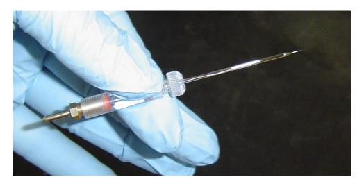
Figure 14: Microelectrode assembly with glass capillary in place.
